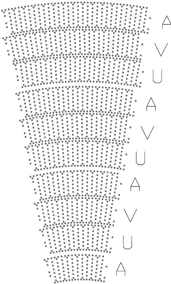
Fig. 2. Cell layout in the BaBar drift chamber.
