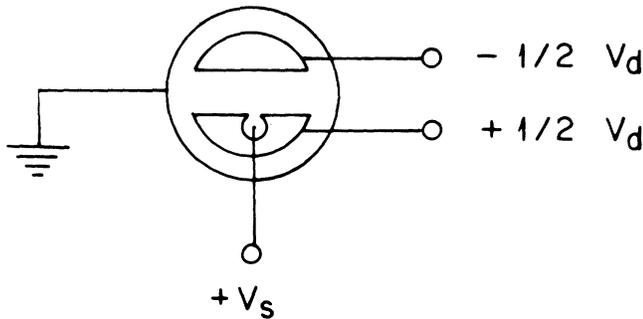
Figure 2 Potentials established in the test chamber
