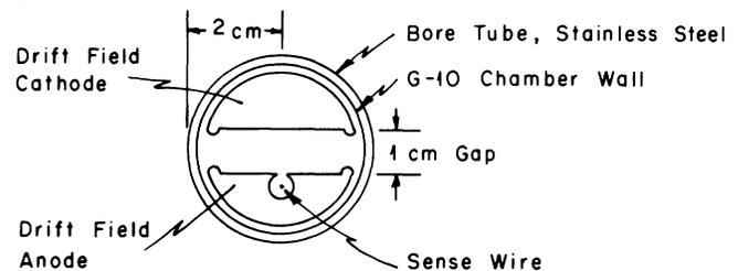
Figure 1 End view of the test drift chamber
