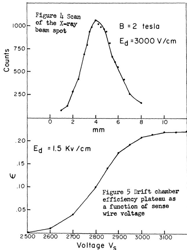
typical plateau for  $E_d = 1.5$  kv/cm as a function of sense wire voltage. For all measured conditions a good operating point was obtained. The chamber performance with the x-ray source was checked by measuring the counting rate as a function of  $V_s$ .
