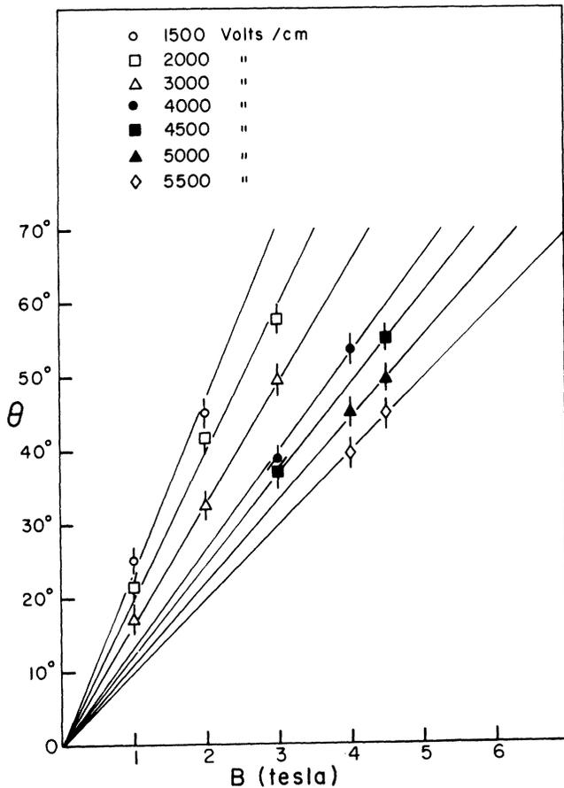
Figure 7 The measured drift angle as a function of the electric drift field and the magnetic field
