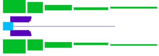
Figure 1: Sketch of the solenoid magnet system around the target. The dark blue rectangles indicate the warm inner coils and the green rectangles indicate the surrounding superconducting coils. The turquoise rectangle is a high magnetization steel pole.
