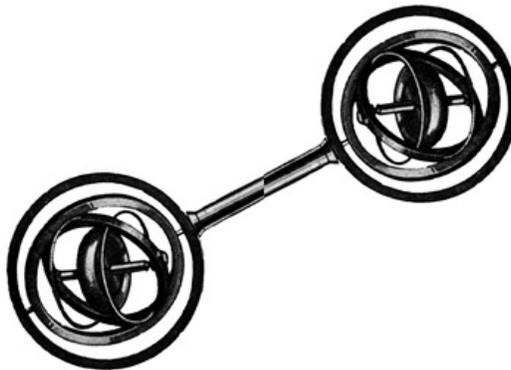
Show that if the spin angular velocity vectors of the two gyrostats are antiparallel, and both lie in the plane of their orbits, then the gyrostats “bob” (oscillate) perpendicular to the plane of the orbit, although the center of mass of the whole system is at rest
