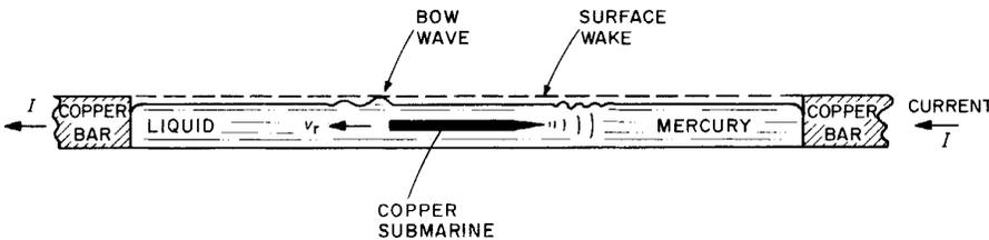
**Fig. 2** Copper submarine experiment. Mercury trough length = 30 cm; cross-section  $0.5 \times 0.5$  inch. Copper extension of troughs 30 cm long,  $0.5 \times 0.5$  inch cross-section. Remote return circuit.  $I = 400$  A. Copper submarine; 5 cm long, 3 mm diameter, 1 cm long taper.  $v_r = 15 \text{ cm s}^{-1}$ .
