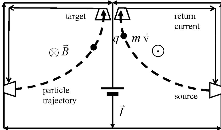
Positive ions are emitted “horizontally” and inwards from sources around a ring on the “vertical” wall of a conducting cylinder, and deflected upwards by the azimuthal magnetic field generated by a “downward” electrical current (driven by a “battery”) in a wire along the axis of the cylinder. When the ions are collected at the (conducting) “top” plate of the cylinder, the latter experiences an impulsive “upward” force.
