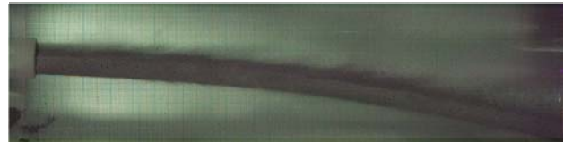
Figure 5. Tungsten powder jet of c.42% material density
